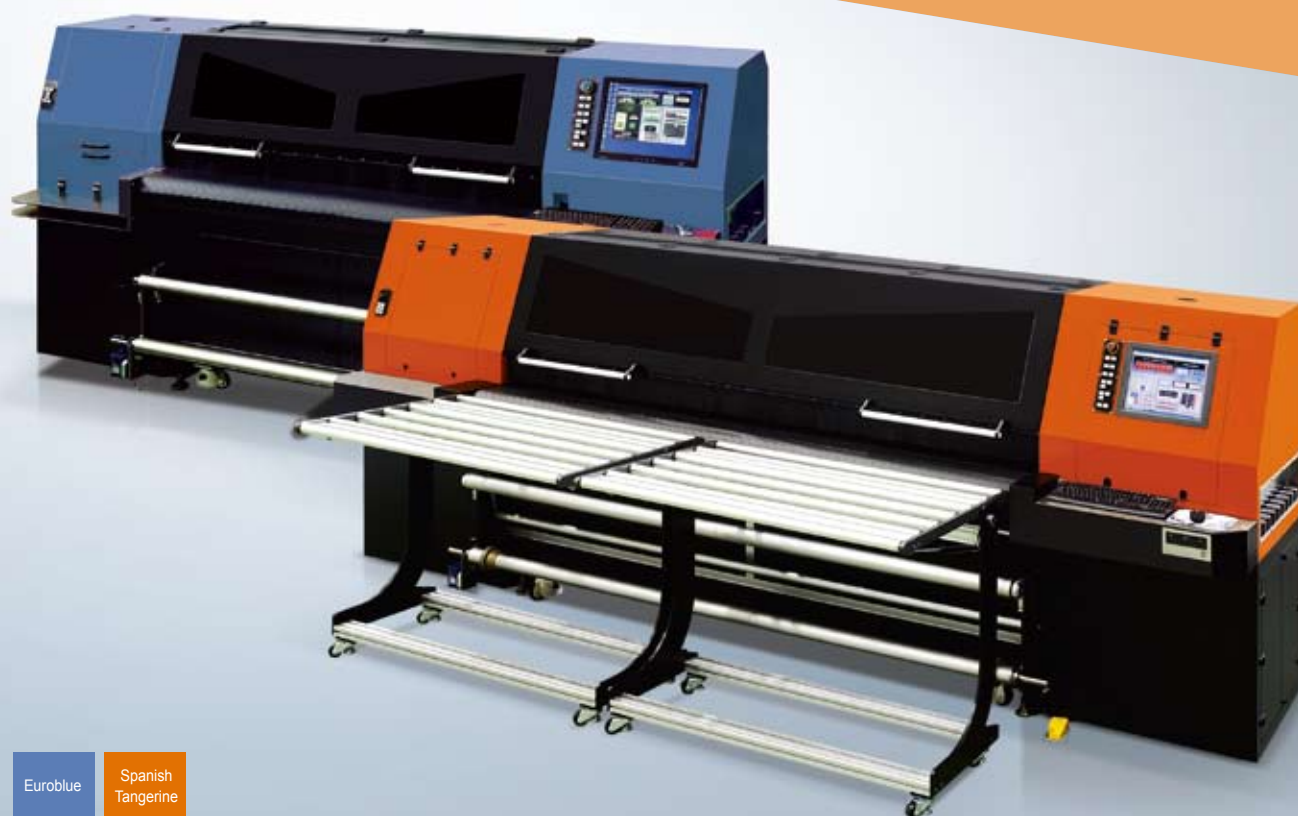
Pop-up extension table for handling small boards and short rolls of flexible materials – no waste on roll media.
