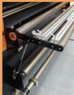
Pop-up extension table for handling small boards and short rolls of flexible materials – no waste on roll media.
