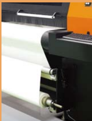
Heavy duty industrial design with idle bar for continuous roll production
