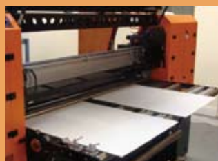
Pin Register System for single or step and repeat multiple boards
